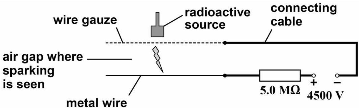
Sparks are produced when alpha particles produce ionisation in the air gap.
