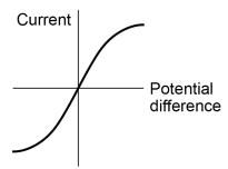
The current through a diode flows in one direction only. The diode has a very high resistance in the reverse direction.
