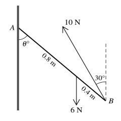
A non-uniform rod AB of weight 6 N rests in limiting equilibrium with the end A in contact with a rough vertical wall. AB = 1.2 m, the center of mass of the rod is 0.8 m from A, and the angle between AB and the downward vertical is  $\theta^{\circ}$ . A force of magnitude 10 N acting at an angle of 30° to the upwards vertical is applied to the rod at B (see diagram). The rod and the line of action of the 10 N force lie in a vertical plane perpendicular to the wall. Calculate
