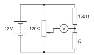
The voltmeter reads 0 V when the slider of the potentiometer is  $\frac{1}{4}$  of the way from its lower end, as shown.
