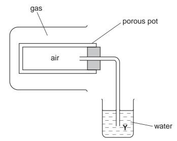
A beaker containing the gas was placed over the porous pot.
