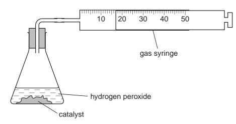
The student carried out two experiments using the same volume of hydrogen peroxide but with the same mass of a different catalyst in each experiment.
