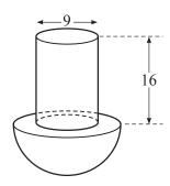
The diagram shows a solid formed by joining a cylinder to a hemisphere. The diameter of the cylinder is 9 cm and its height is 16 cm.
