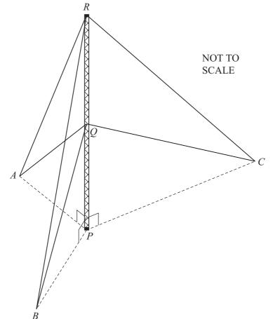
The diagram shows a vertical radio mast *PQR* supported by 6 straight wires.
