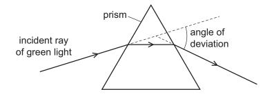
When a ray of white light is incident on the prism, it separates into the colours of the visible spectrum.
