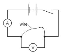
When the switch is closed, the ammeter reads 2A and the voltmeter reads 10 V.
