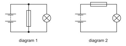
A fault develops. The current in the lamp increases, and the fuse blows.
