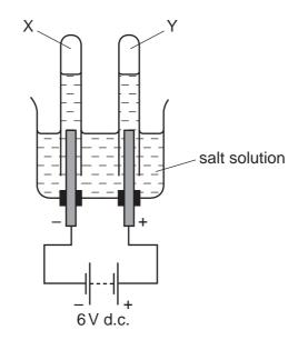
One of the gases explodes when tested with a burning splint and the other turns moist Universal Indicator paper red then white.
