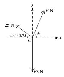
Three horizontal forces of magnitudes F N, 63 N, and 25 N act at O, the origin of the x-axis and y-axis. The forces are in equilibrium. The force of magnitude F N makes an angle  $\theta$  anticlockwise with the positive x-axis. The force of magnitude 63 N acts along the negative y-axis. The force of magnitude 25 N acts at  $\tan^{-1} 0.75$  clockwise from the negative x-axis (see diagram). Find the value of F and the value of  $\tan \theta$ .
