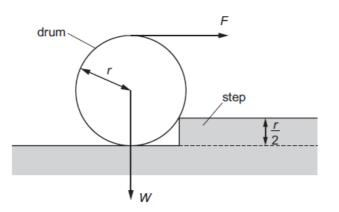
What is the minimum force *F* required for the drum to start rolling on the step?
