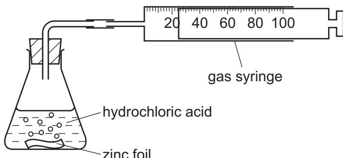
A piece of zinc foil was added to  $50\text{ cm}^3$  of hydrochloric acid, of concentration  $2.0\text{ mol/dm}^3$ . The acid was in excess. The hydrogen evolved was collected in the gas syringe and its volume measured every minute. The results were plotted and labelled as graph 1.
