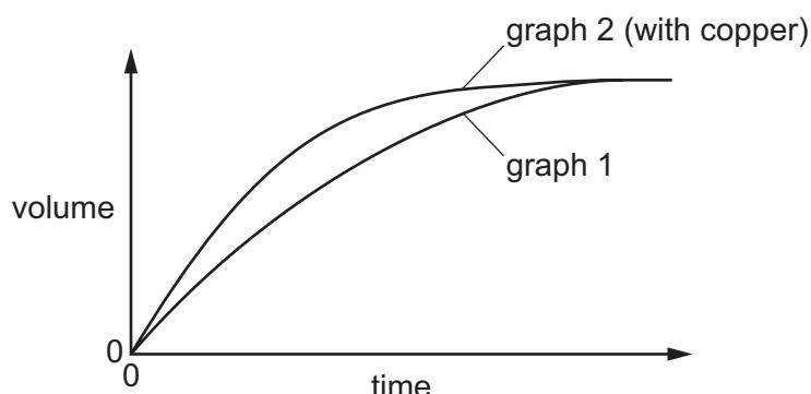
The experiment was repeated to show that the reaction between zinc metal and hydrochloric acid is catalysed by copper. A small volume of aqueous copper(II) chloride was added to the acid before the zinc was added. The results of this experiment were plotted on the same grid and labelled as graph 2.
