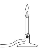
(a) The Bunsen burner uses methane as a fuel.
