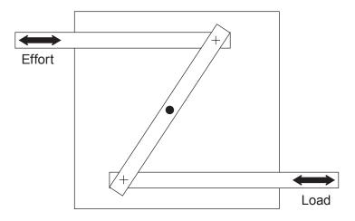
Complete the linkage system below using  $\bullet$  for fixed pivots and + for moving pivots to achieve the desired movements with a velocity ratio (VR) of 1:2. [3]
